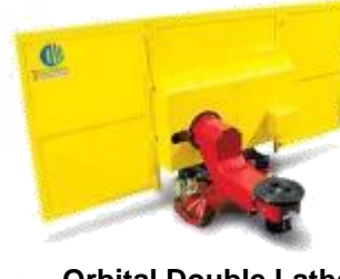
Orbital Double Lathe Payload: 250 ÷ 750 kg Available "single lathe"
